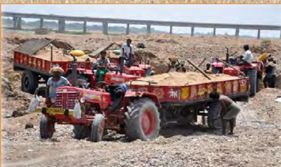
On the Tungabhadra riverbed at Panchalingala village in Kurnool district, Andhra Pradesh, sand is collected in tractor trailers fitted with sieves. In the background is National Highway 7. Photo: U. Subramanyan
