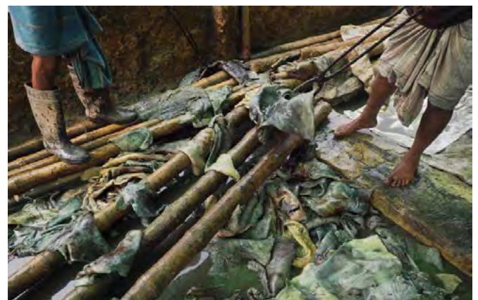
Raw hides soaked in lime and sodium sulphide to remove hair and fat.
