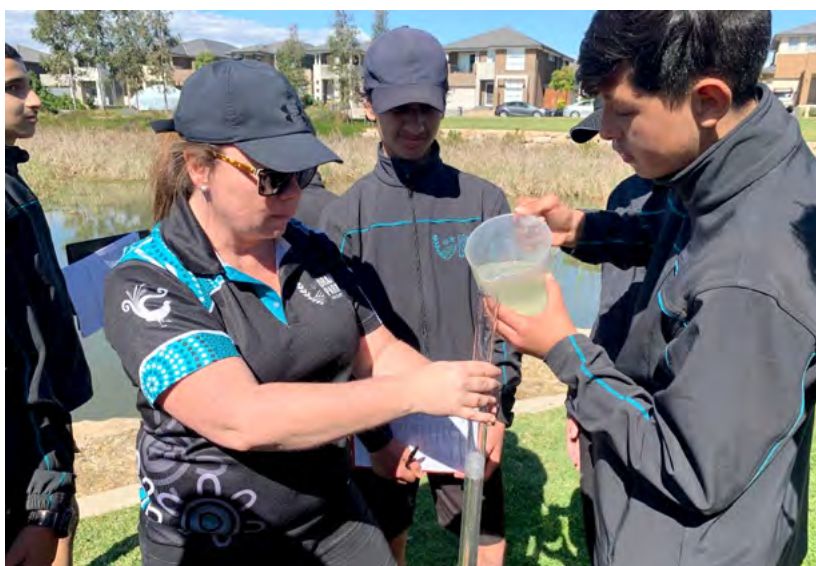
Figure 11: Using a turbidity tube to measure turbidity of the stormwater.
