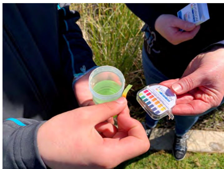
Figure 12: Using universal indicator paper to determine stormwater pH level.
