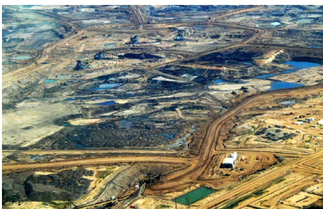
Figure 20: Excavation of oil sand at Fort McMurray in Alberta, Canada. The Athabasca oil sands deposit is among the largest in the world. The bitumen contains lots of hydrocarbons but is notoriously hard to extract. It is only economically viable when world oil prices are high. It also makes a major contribution to Canada's greenhouse gas emissions. Source: Wikimedia Commons
